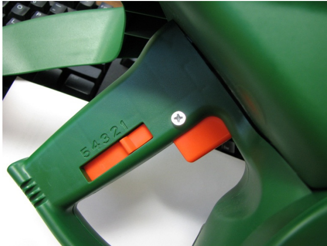
Screw holding the trigger permanently open.
